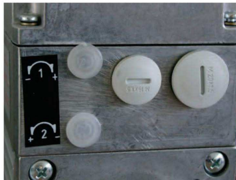
Adjusting screws for the operating range and maximum range detectors
