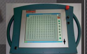
The automation system commander can be used as an control system both local and central. On demand, an access can be realised for remote support (remote maintenance).
